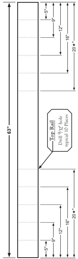
Alternate method of fabricating a Small Goal
